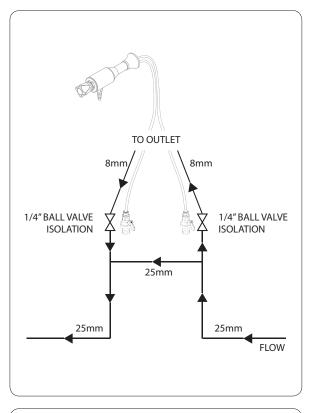
Flow / Return Circulating System (Optimum Installation)
