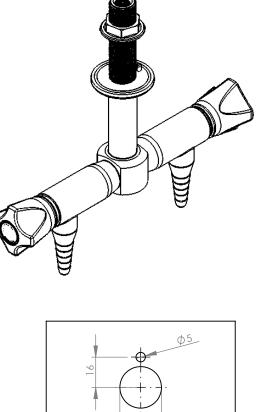
Ø22 INSTALLATION DETAIL (WALL CUTOUT) PLEASE CHECK LOCKING PIN POSITION BEFORE INSTALLATION AS ORIENTATION MAY VARY
