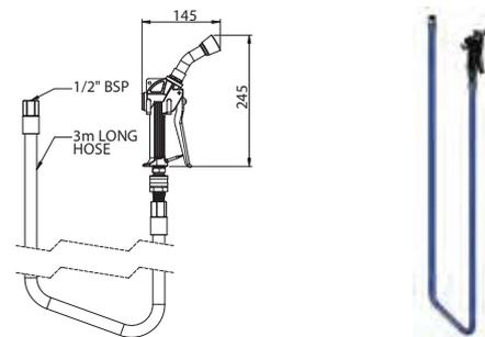
**Hot & Cold Wash Down Hose Reel with FS731 Delrin Trigger Spray**
