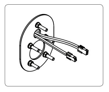
6. Seal edge of front plate with silicone sealant to finish off the installation.(Use anti-pick silicone or silicone sealant of appropriate grade as required.)
