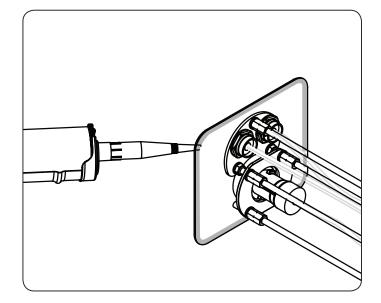
4. Fit control plate into position.
