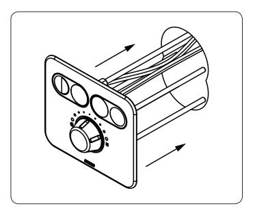
5. Feed cables through. Attach rear plate and secure with nut and washer sets.
