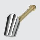
Tubular style anti-ligature shower rose either wall mounted or duct mounted with anti-rotation pin and torx security grub screw for added safety.
