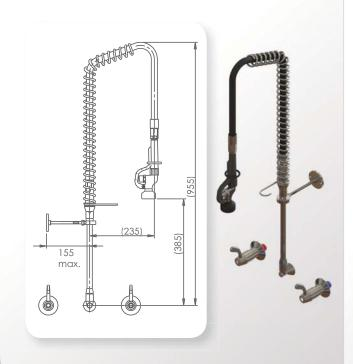
WALL MOUNTED PRE-RINSE UNIT WITH CONCEALED MIXER ASSEMBLY WITH A POT FILLER
