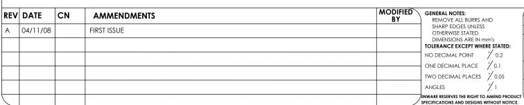
GENERAL NOTES: REMOVE ALL BURRS AND SHARP EDGES UNLESS OTHERWISE STATED DIMENSIONS ARE IN mm's TOLERANCE EXCEPT WHERE STATED: NO DECIMAL POINT ONE DECIMAL PLACE TWO DECIMAL PLACES
